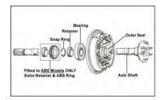
This diagram explains the set-up of rear wheel bearing half shaft found on the Toyota  $4\times4$  rear axles with and without ABS.
