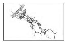
Remove inner axle oil seal.
