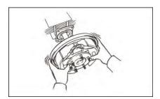
Remove the wheel and brake drum; disconnect the brake tube and hand brake cable.
