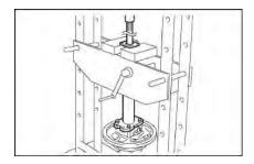
Using a press, press out the rear axle shaft from the backing plate.
