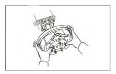
Install the rear axle shaft with four nuts and Torque to 700kg-cm (51 ft-lb, 69N-m). Be careful not to damage the oil seal.
