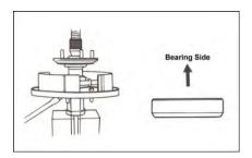
Insert the backing plate and bearing retainer on the rear axle shaft.
