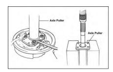
Using a **Rear Axle Shaft Puller (Pt No. TOOL1)** attach it to the backing.
