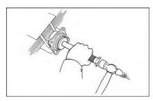
Clean surfaces and install new inner axle oil seal being carefull not to damage the new seal.
