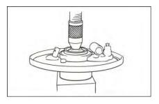
Inspect the rear axle bearing for wear or damage.
