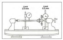
Maximum shaft runout: 2.0mm (0.079 Inch) Maximum flange runout: 0.2mm (0.008 Inch)
