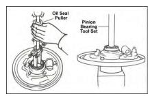
Inspect the oil seal for damage and check the oil seal lip for wear or damage.
