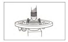
Inspect bearing case and clean all surfaces with emery cloth and press the new bearing into the hub. Install new oil seal.
