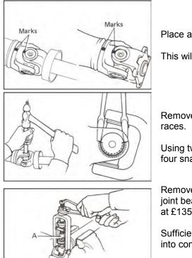
Place alignment marks on the shaft and flange or yoke.
